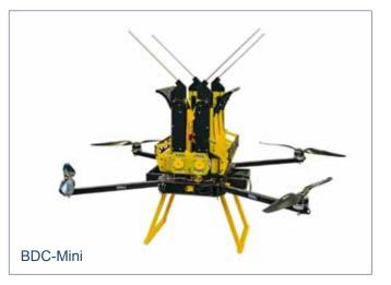
aircraft, with most parts 3D printed for easy replacement in case of crashes.
