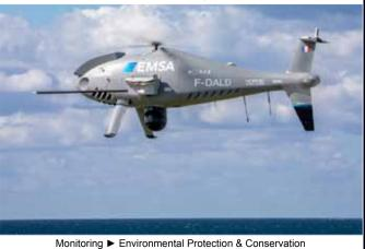
Monitoring ► Environmental Protection & Conservation ► Pollution (aerial, maritime, terrestrial) Camcopter S-100 monitoring ship sulphur emissions for EMSA - Schiebel, Austria
