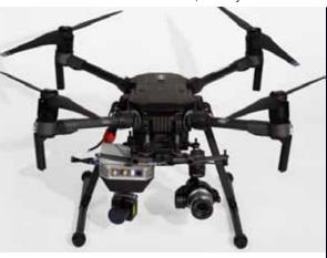
Drone for aircraft fuselage inspection Maintenance Mainblades, The Netherlands
