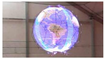
Spherical Drone with Projection on Exterior (indoor flight) NTT - Docomo, Japan
