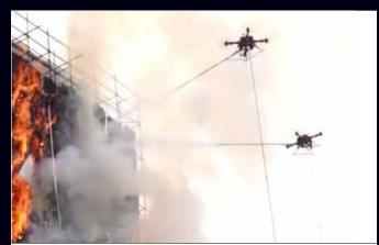
Fire Fighting ▶ Public Services & Safety ▶ Urban fire ▶ Extinguishing High-Rise Fire Fighting Drone Chongqing Guofei General Aviation Equipment Manufacturing, China (PR)
