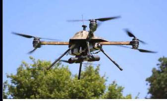
Manipulation ► Security & Law Enforcement ► UXO clearance (disruptor) Protector - Steelrock Technologies, UK
