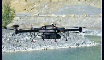
Inspection ► Environmental Protection & Conservation ► Hydrography ► Bathymetric BathyCopter - Riegl Laser Measurement Systems, Austria
